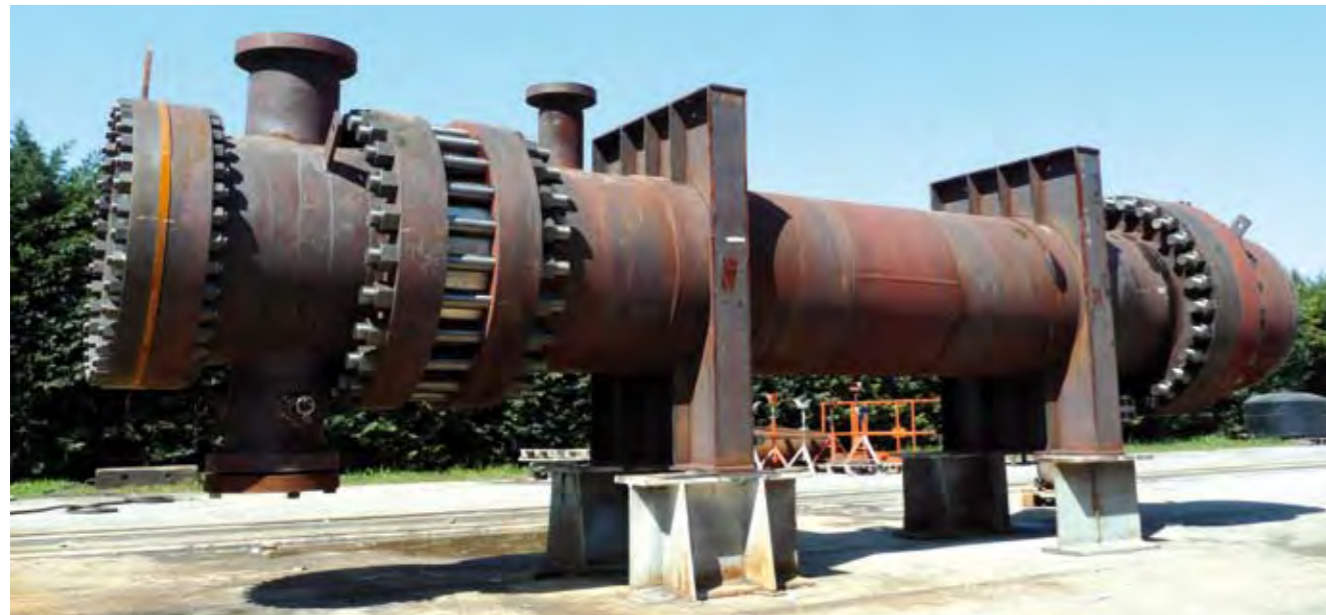
PROJECT CLIENT / END USER M-3401D Reactor Effluent/Fresh Feed Exchange Hellenic Petroleum s.a., Aspropyrgos Refineries
