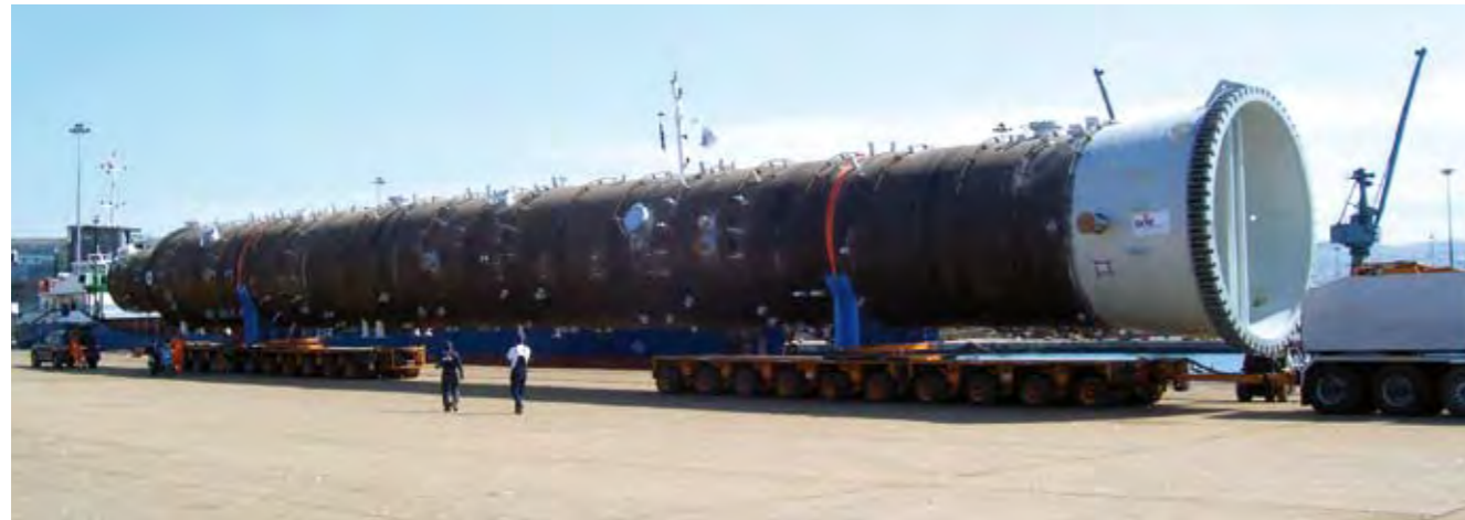
PROJECT CLIENT END USER C-7102_ Crude Fractionation Column Technipetrol Hellas S.A. Motor Oil (Hellas) Corinth Refineries s.a.
