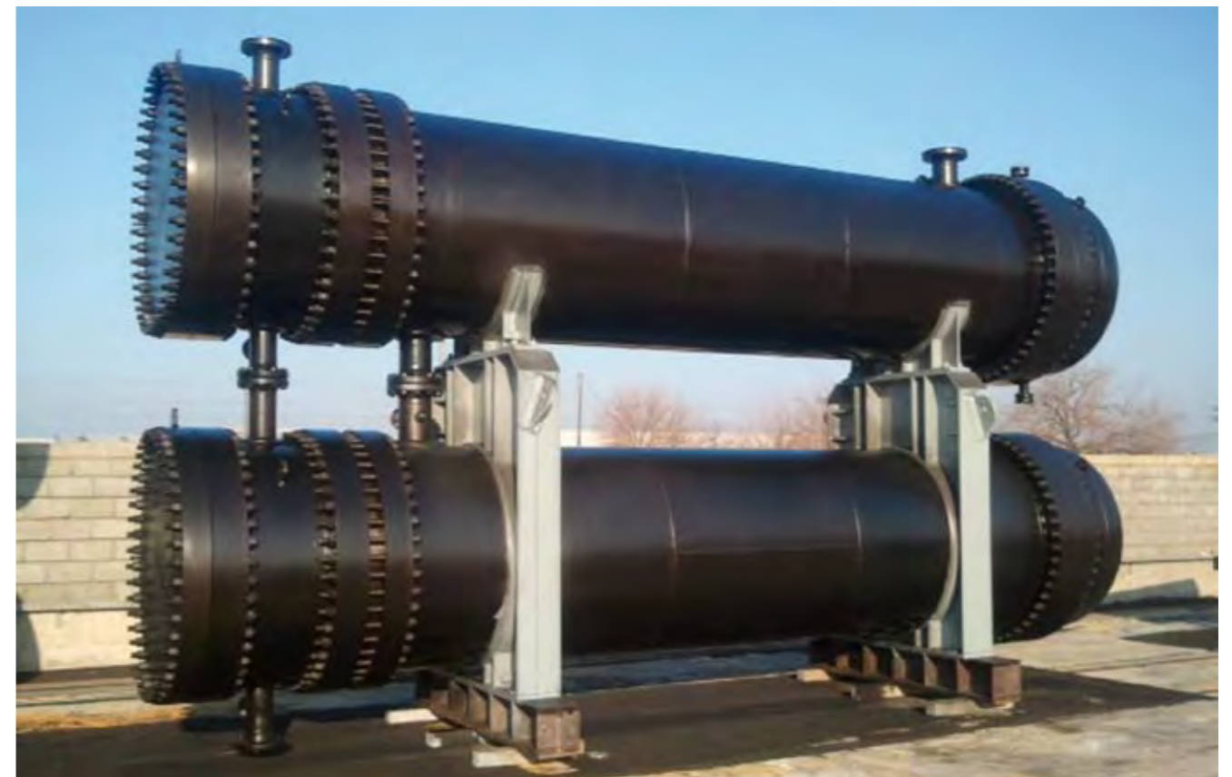
PROJECT: CLIENT / END USER S&T C.S. Heat Exchangers - VDU Unit Elefsis Refinery Upgrade Project Hellenic Petroleum s.a., Elefsina
