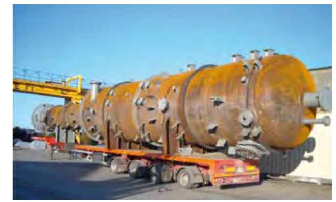
PROJECT CLIENT / END USER Outboard Flash Tower T150 Hellenic Petroleum s.a., Thessaloniki Refinery
